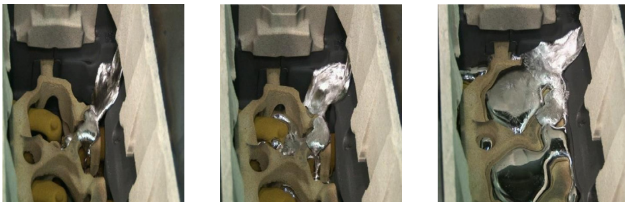
Figure 3. Change in flow direction during the mold filling process of a cylinder head: The cover core was modified to allow high-speed videos of the melt flowing from the runner through the gates to be taken.
