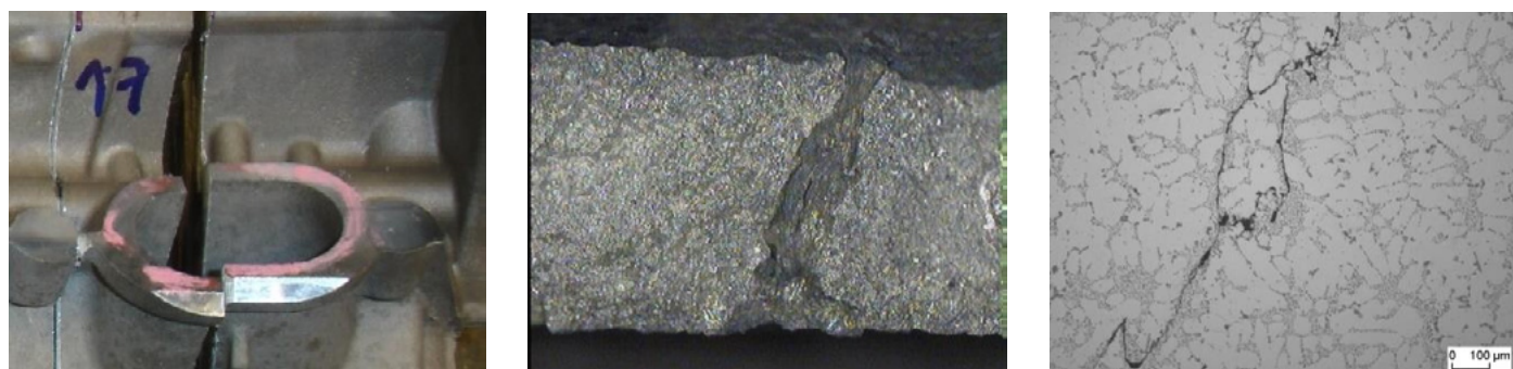
(a) Cut through leaking cylinder head (b) Fracture analysis through leaker (c) Microstructure analysis
