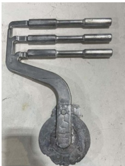
Figure 2- Tensile bar die casting. Hot shear specimens were taken from the middle-reduced section of the tensile bars.
