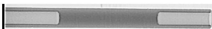
Figure 3- X-ray image of shear specimen showing a porosity free center testing region. The light regions of either end of the specimen are the bores for the insertion heaters.
