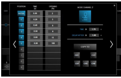
3.3 Illustration: The setting of the throttle valve to reduce the air flow.
