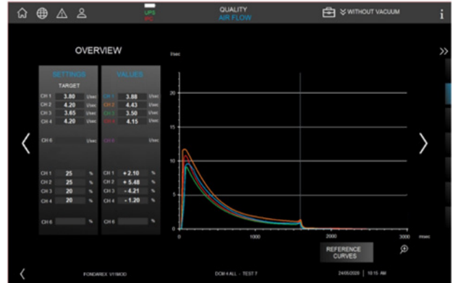
3.6 Illustration: The measurement of the air flow moved in each vacuum port
