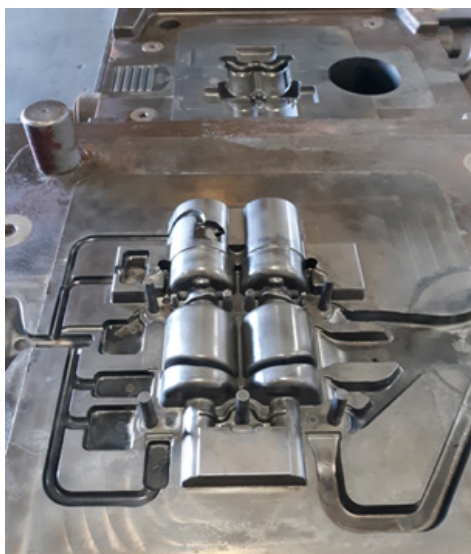
Figure 4: Photographs of both the fixed and moving side of the AlCrN PVD coated balance shaft housing die after 100,000 shots [6]
